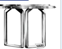
Figure 1. Two rectangular stirrers that rotate on their own axes as hey revolve on a common axis move through the batch continuously mixing materials up to about 2 million cP.
