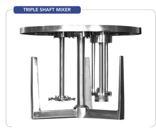
Figure 4. The 3-wing anchor stimulates greater flow in the mix vessel and moves material toward two stationary high-shear agitators, increasing their effective viscosity range.
